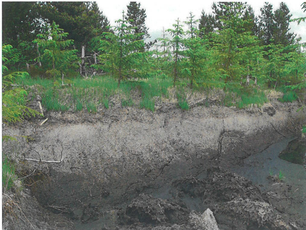
Figure 1. Smooth face of a peat crack, or fissure, resulting from peat shrinkage caused by water loss from the peat matrix as a result of drainage. The face is aligned along a former forestry ploughing furrow. Photograph taken during a 2004 field investigation of the Derrybrien windfarm site.
